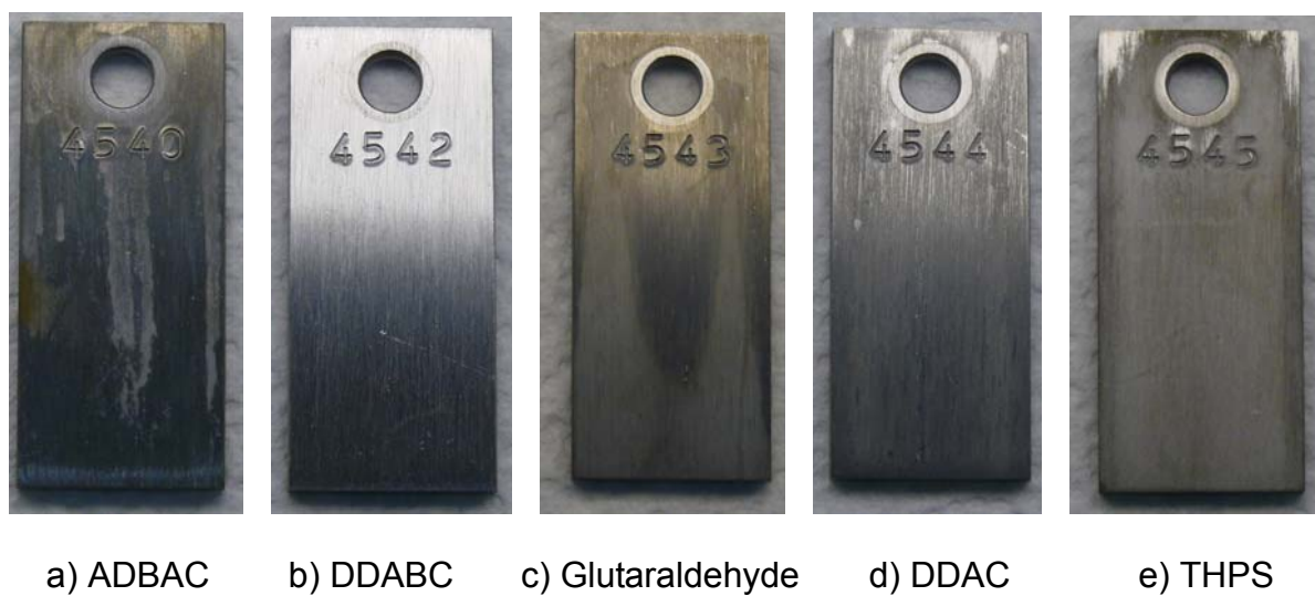
Figure 3 - Autoclave Test Coupons from result reported in Table 4
